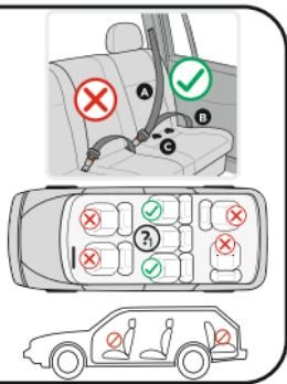
**INSTALLATION OF SEAT WITH 3-POINT SEAT BELT + FIX ATTACHMENT.**
